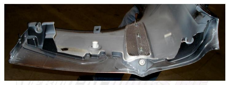
The fender side vent will have to be modified in order for the VDI kit
