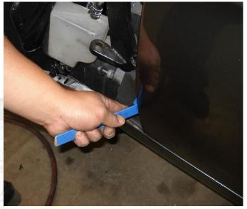
Also make sure to measure the distance from the body to the edge of the door. This will ensure that the door and fender meet like factory once you install the new VDI kit.
