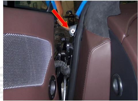
Remove the weather stripping from around the bottom of the door. This will give you access to the top side skirt bolts that hold the fender and side skirt in place.
