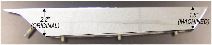
Put the fender back together and test fit the fender to the car. Make sure there is no contact between the VDI Hinge and the fender side vent. After make sure the kit works properly. Replace the fenders making sure to match up the factory marks in step 3.
