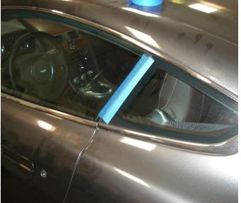
Make sure to mark the factory door position on the vertical and horizontal planes.
